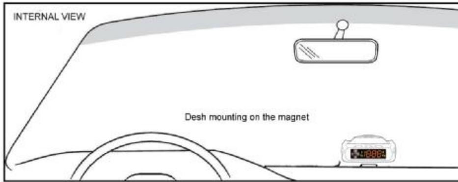
**Where to mount GPS & radar detector**
