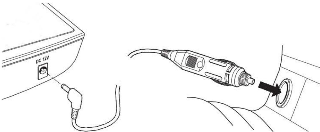
The **GPS & radar detector** operates on 12 volts DC negative ground only. The power cable provided is a standard size and will work in most vehicles. However, some vehicles may require our optional sleeve to ensure a snug fit. If so, simply call or contact with local dealers.
