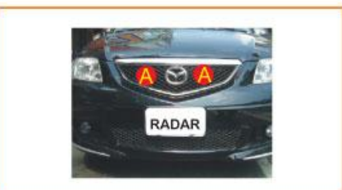
Installation on A or B inside Bumper Extension if no Chrome Trim
