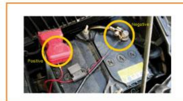
The negative pole first installation and then the positive electrode
